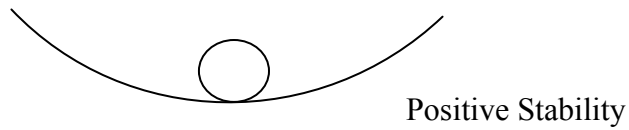
Figure 4.12 – Positive Metacentric Height
